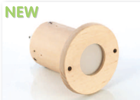
LED-installation-light single coloured white 5.5 W for sauna up to 110 °C and bio-sauna art. no. 71051
